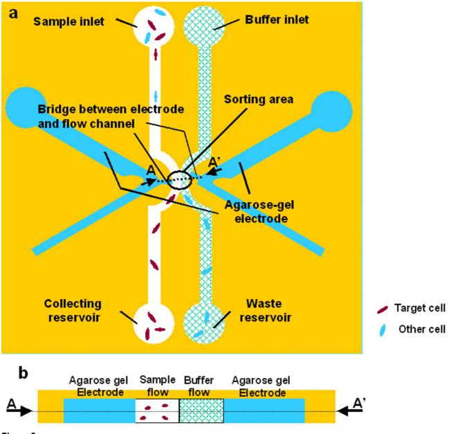
**Figure 2** Whole structure of on-chip cell sorter.
