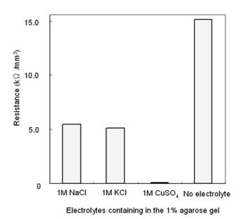
Figure 7 Electrolyte dependence of 1% agar gel resistances ( $\Omega/\text{mm}^3$ ).
